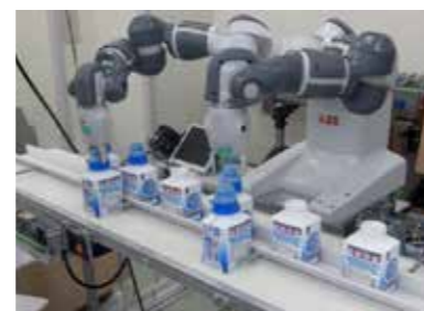
Robotics used to temporarily tighten bottle caps
