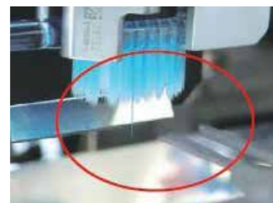
The automated bristle inspection and removal system that duplicates the craftsmanship achieved to date through human hands
