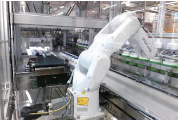
Automated dental rinse bottle supply using robots
